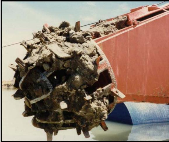
A sand & gravel screening style cutter basket plugged with clay and near-size material.
