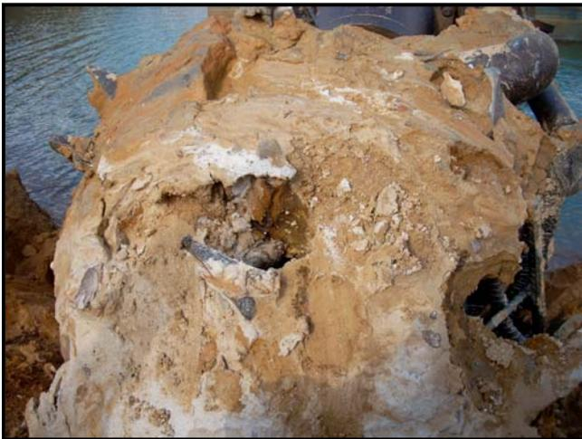
A typical bladed style cutter basket with sizing bars completely choked with clay and near-size material.
